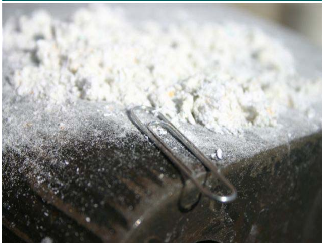
The new NFPA standard of 1/32" in accumulated dust thickness is all it takes to be out of compliance.
